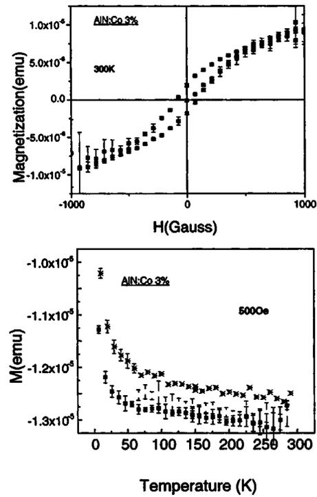
FIG. 4. 300 K magnetization as a function of field (top) and FC and ZFC magnetization as a function of temperature (bottom) for AlN implanted with  $3 \times 10^{16} \text{ cm}^{-2} \text{ Co}^+$  and annealed at  $950^\circ\text{C}$ , 2 min.
