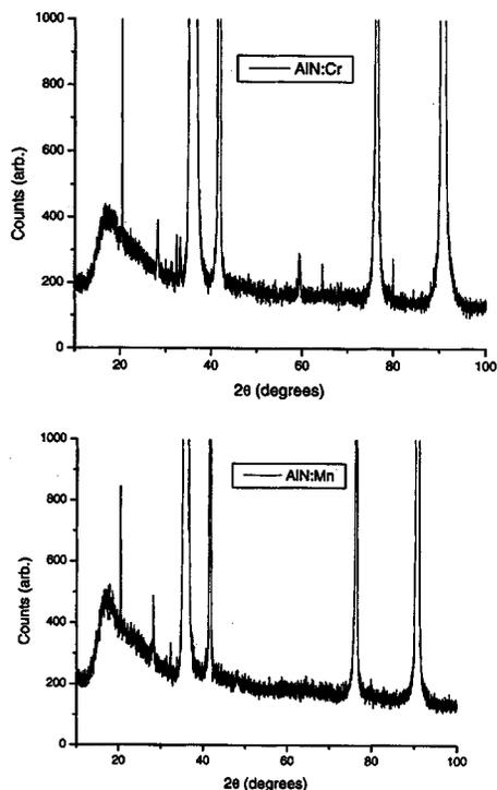
FIG. 6. X-ray diffraction scans of AlN implanted with  $\text{Cr}^+$  (top) or  $\text{Mn}^+$  (bottom) to a dose of  $3 \times 10^{16} \text{ cm}^{-2}$  and annealed at  $950^\circ\text{C}$ , 2 min.
