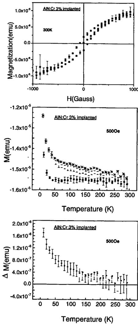
FIG. 3. 300 K magnetization as a function of field (top), field-cooled (FC), and zero-field-cooled (ZFC) magnetization vs temperature (center) and difference in FC-ZFC magnetization vs temperature for AlN implanted with  $3 \times 10^{16} \text{ cm}^{-2} \text{ Cr}^+$  and annealed at  $950^\circ\text{C}$ , 2 min.
