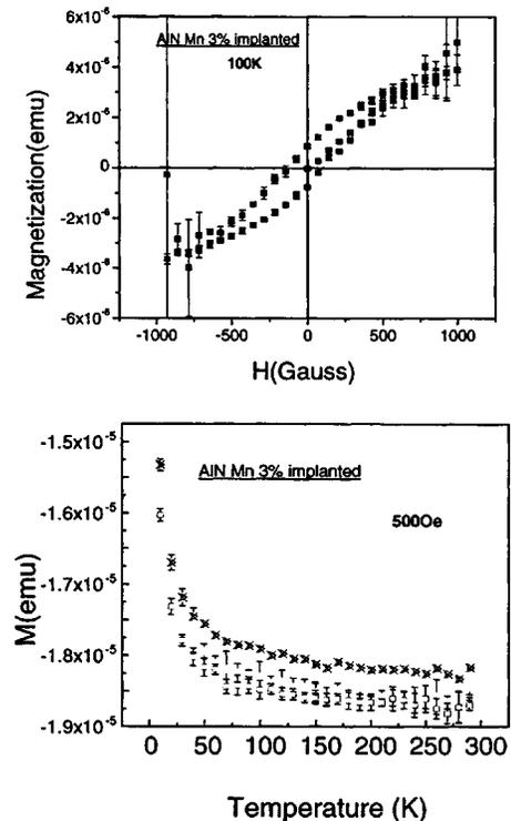
FIG. 5. 100 K magnetization as a function of field (top) and FC and ZFC magnetization as a function of temperature (bottom) for AlN implanted with  $3 \times 10^{16} \text{ cm}^{-2} \text{ Mn}^+$  and annealed at  $950^\circ\text{C}$ , 2 min.
